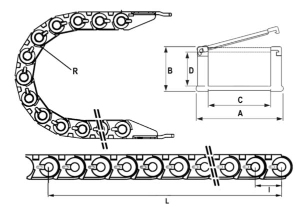
Full length = 1008mm Inside Height = Inside Width = Link Length(Pitch) = Outside Height = Outside Width = Radius = 150
